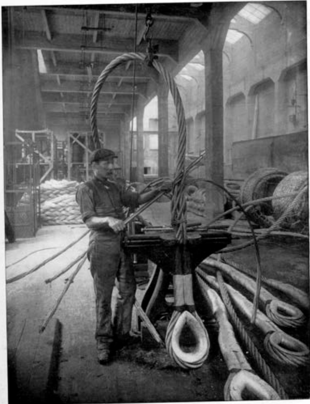
Splicing a set of Launching Checks, 8in. circ., of a total length of 4,500 feet, having a guaranteed test breaking stress of 200 tons, at THOS. & WM. SMITH Ltd., Wire Rope Manufacturers GUILDHALL, NEWCASTLE-ON-TYNE
